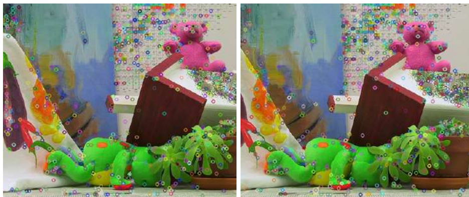
Figure 4.3: Example of one pair of images after applying the SIFT algorithm.
