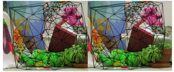
Figure 6. Delaunay Triangulation of a set of corresponding points using the Teddy stereo par.
